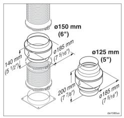
In some cases, a condensate trap may also be required to collect and evaporate any condensate which may occur. This optional accessory is available for ducts 5" (125 mm) and 6" (150 mm) in diameter.
